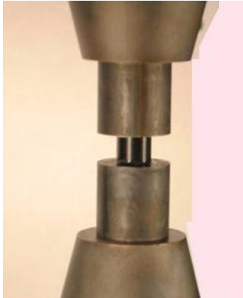
Figure 3.10: Setup of a compression test
