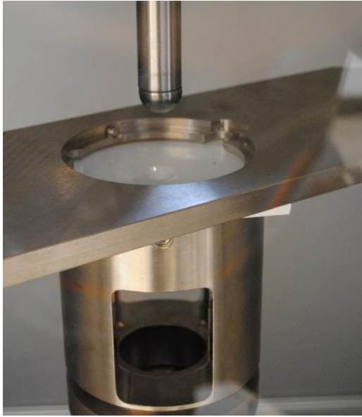
Figure 5.40: The plate and the shaft right after impact.
