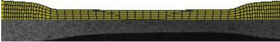
Figure 5.3: Propagated necking in tensile specimen T1, comparing experimental and simulated neck.
