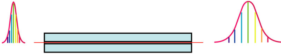
Figure 18: Chromatic dispersion in a fiber[14]
