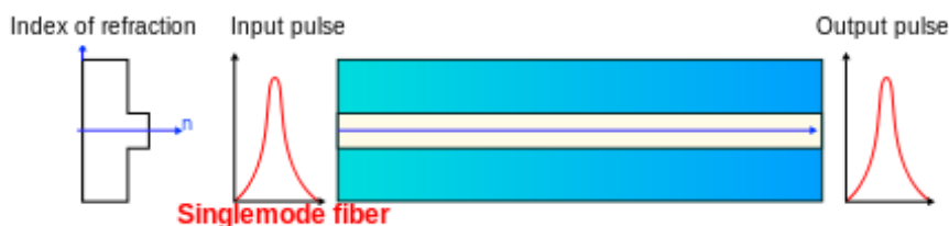
Figure 12: Light propagating through singlemode fiber[25]
