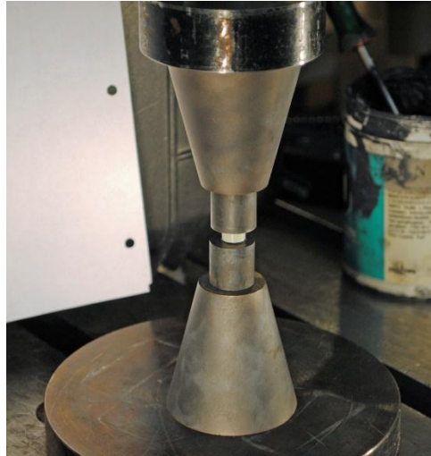
Figure 3-23. Test setup for compression tests.
