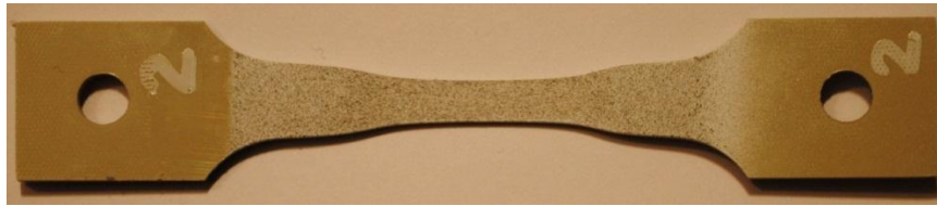
Figure 3-16. Test specimen after a the testing, with a deformation of 46 mm.
