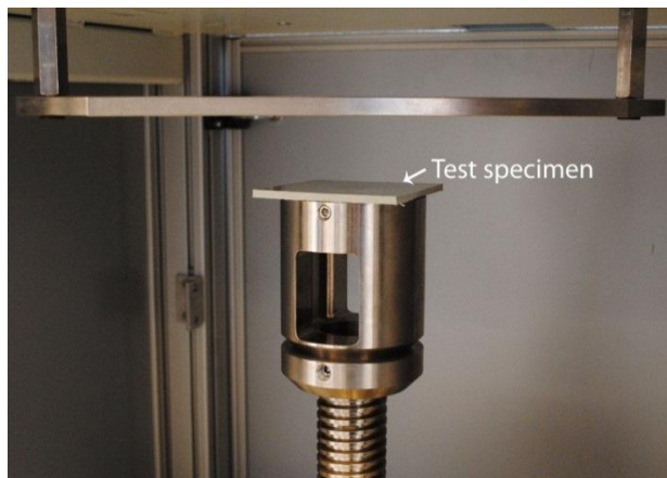
Figure 6-17. Test setup in the Drop Tower machine.
