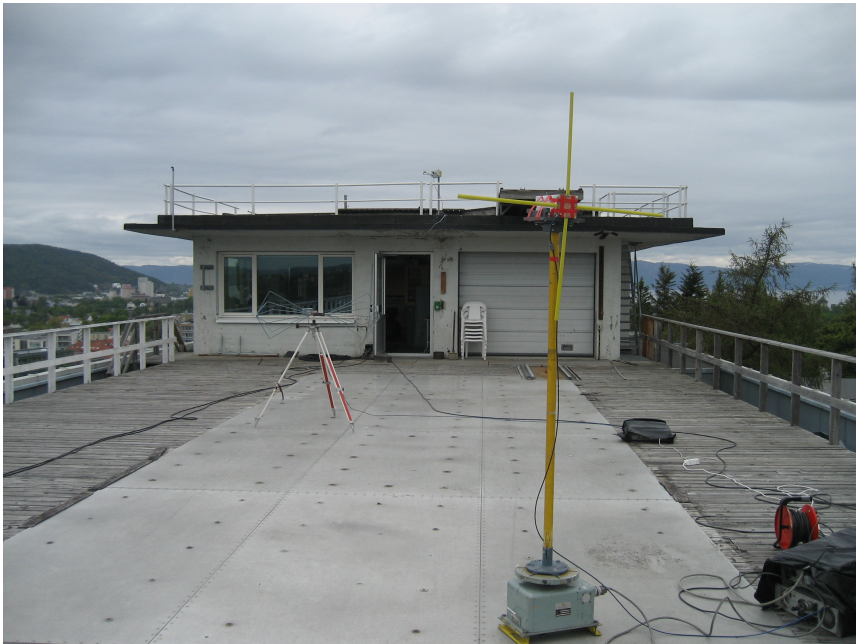
Figure 10.6: The test range. The range is placed at an angle to lower specular reflections from the wall.
