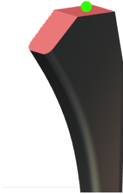
Figure 24: Reference point (green), fully constrained to the femoral neck region (red).
