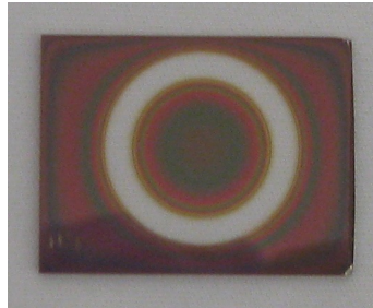
Figure 3.4.1: Glass plate gone through PECVD with part of it covered. It is evident that the growth profile is uneven.
