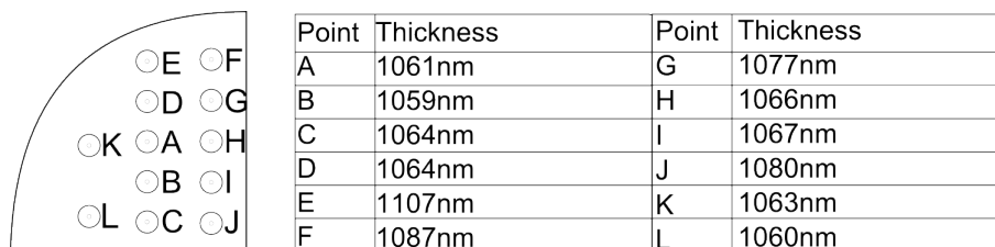
Figure 4.2.7: Refractometer measurements for the SiO_2 layer with \sim 1060 nm thickness.
