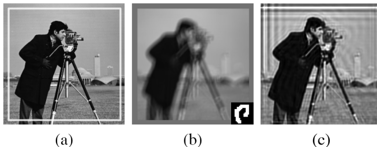
Figure 4.10: Illustration of typical boundary artefacts, from [31]. (a) The original image with field of view within the white lines. (b) Blurred image padded with mean values along the boundaries. (c) Restored image with boundary artefacts.
