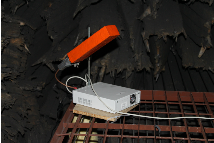
Figure 1: Ettus Research USRP2 with a horn antenna mounted on a custom made antenna stand.
