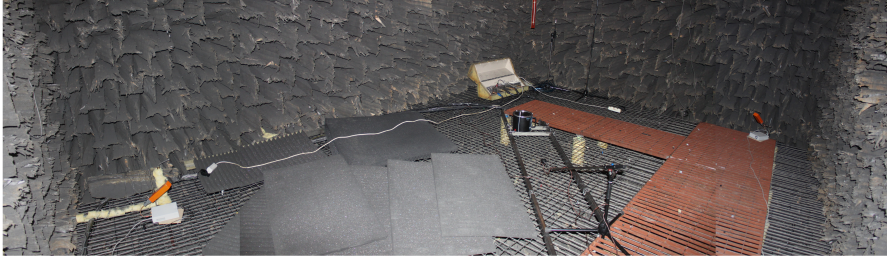
Figure 7: An image composed of three pictures, showing the entire bistatic RASS, setup A in the anechoic chamber.
