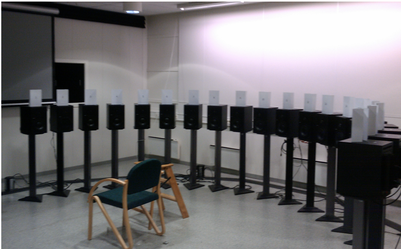
Figure 4.1: Picture of the loudspeaker setup in the listening room. The white squares are paper sheets with numbers ranging from 1-19.
