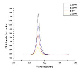
Figure 4.4: Pulsed laser illumination, 310nm, NW2
