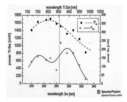
Figure 3.4: FHG tuning curve,  $3\omega$ , 10 W pump laser
