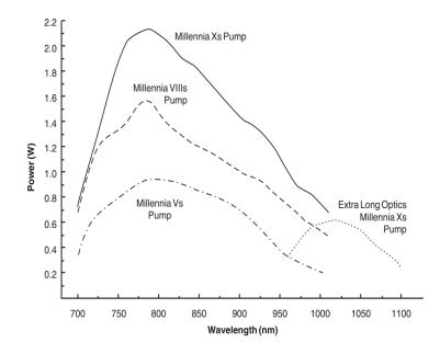
Figure 3.3: Tsunami femtosecond tuning curves for broadband optics when pumped by the various Millennia diode-pumped lasers shown.
