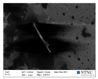
Figure 3.1: SEM image of a dispersed wire
