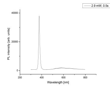
Figure 4.1: PL spectrum of NW1, continuous wave
