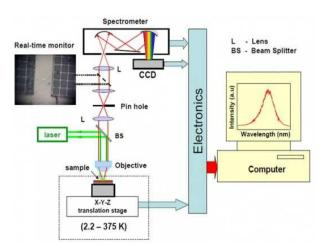
Figure 2.2:  $\mu$ -Photoluminescence spectroscopy setup
