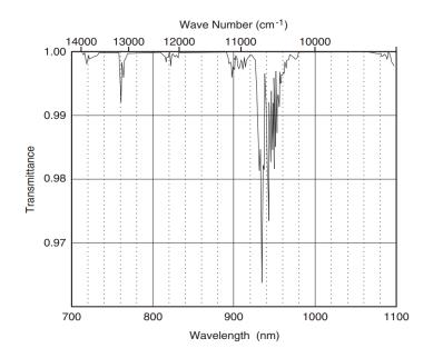
Figure 3.2: Transmittance vs Wavelength for Oxygen and Water Vapor
