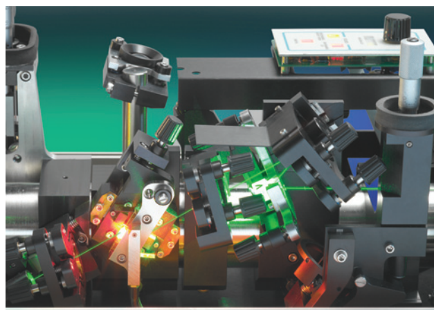
Tsunami HP high-performance optics offer the broadest tuning range of 700 to >1080 nm
