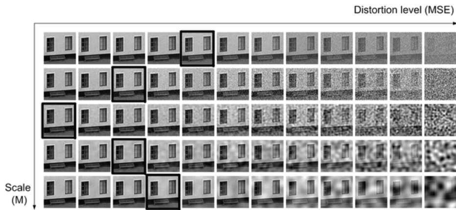
Figure A.8: Demonstration of the table of distorted images. Images in the same column have the same MSE. Images in the same row have distortions only in one specific scale. Each subject was asked to select a set of images, one from each scale, exhibiting similar visual qualities. As an example, one subject chose the marked images.
