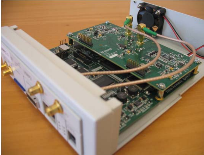
Figure 6. Opened USRP2 platform.
