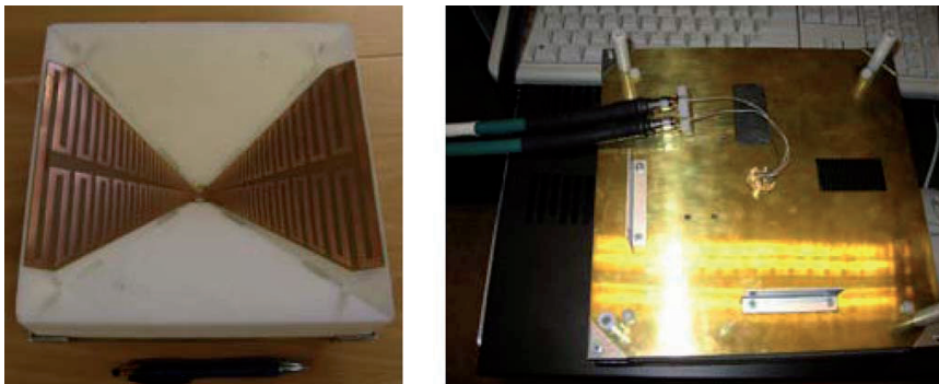
Figure 6.17: Eleven feed for 1-10 GHz (21-pair dipoles) and the measurement set-up for reflection coefficient [2].
