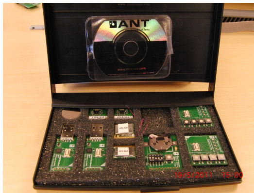
Figure 34: ANT development kit. The modules labeled AP2-1CH and AP2-8CH were used in this project. The 8-channel device was connected to one of the USB modules and plugged in a PC.
