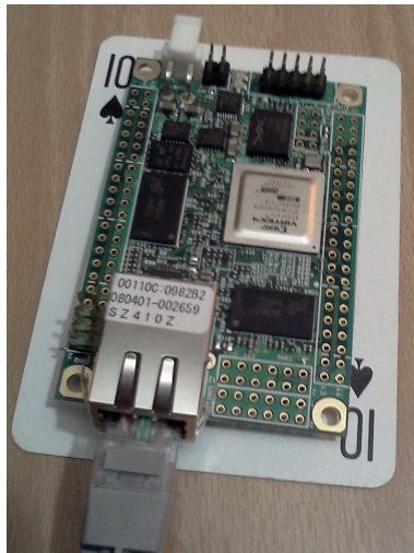
Figure 3.2: The Suzaku-V development board from Atmark-Techno.
