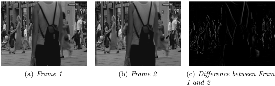
Figure 2.11: Two consecutive frames in a video of people walking down a street and the difference between them. The entropy in both the frames is about 6.75 bits/pixel while it is about 2.5 bits/pixel in the difference image
