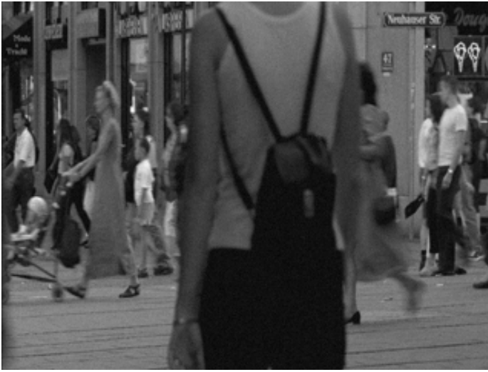
Figure A.17: From from TV1 for the 3d-dpcm-case. E_p/N_0 = 3 dB, PSNR = 40 dB
