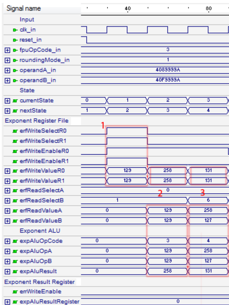
Figure 4.3: Floating-Point Multiplication: Exponent Calculation
