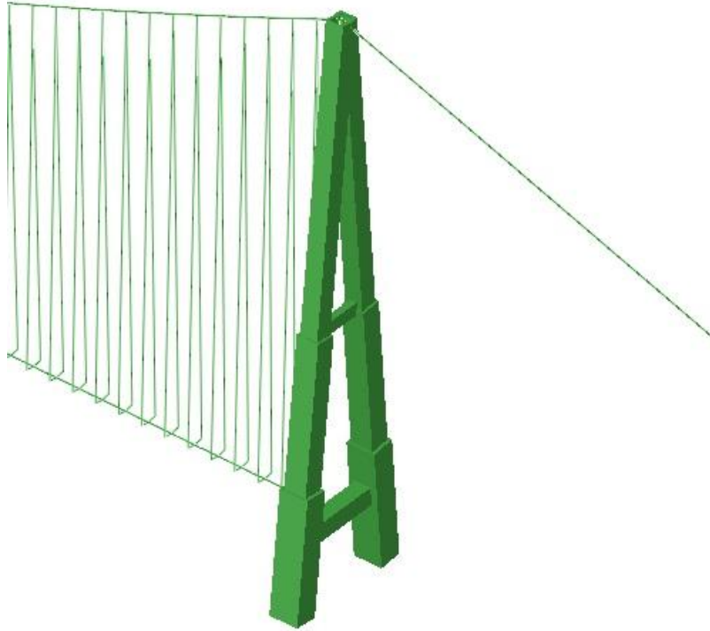
Figure 3.6 Pylon for a mono-cable suspension bridge.
