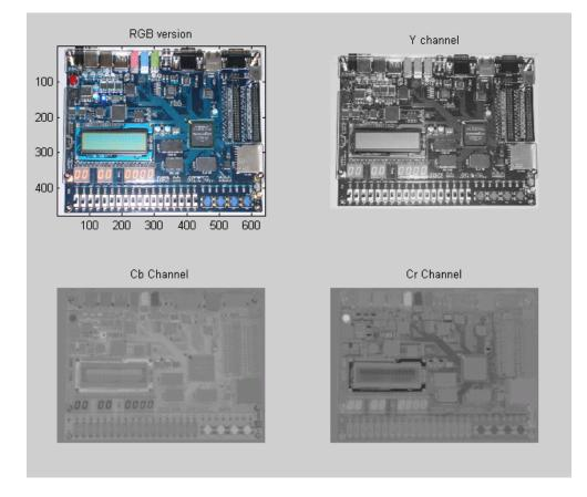
Figure 4.2: A YCbCr color image and its channels
