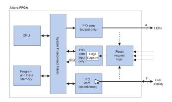
Figure 7.1: NIOS II sample system with multiple PIO cores - from [21]
