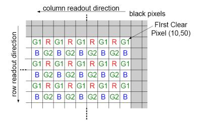
Figure 4.4: Pixel color readout pattern (Bayer) - from [56]
