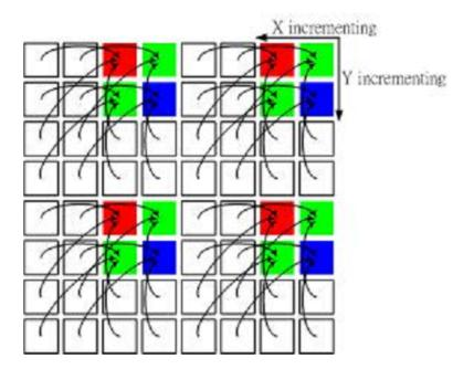
Figure 4.6: 2X binning on Terasic D5M - from [56]
