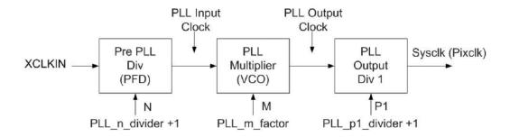
Figure 6.6: Shows how the camera's PLL is implemented - from [56]
