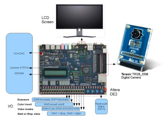
Figure 10.1: An overview of the demonstrator and its I/O
