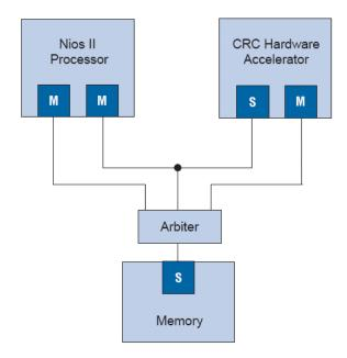
Figure 3.3: Example of a CRC Hardware Accelerator with Nios II - from [19]
