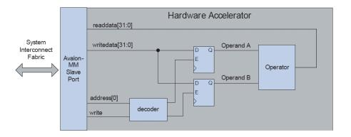
Figure 3.4: Example of a Hardware Accelerator - from [19]
