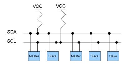
Figure 7.3:  $I^2C$  bus system - from [30]
