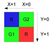
Figure 9.7: A group of four pixels in mirror readout pattern
