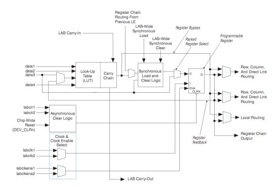
Figure 6.2: Logic Element in Cyclone II - from [13]
