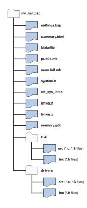
Figure 5.1: HAL BSP After Generating Files - from [20]
