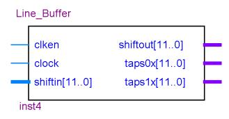
Figure 9.8: The Line-buffer used by both hardware and software for color interpolation
