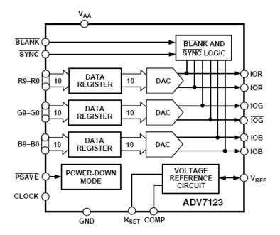
Figure 6.3: Functional Block diagram of the VGA DAC - from [26]
