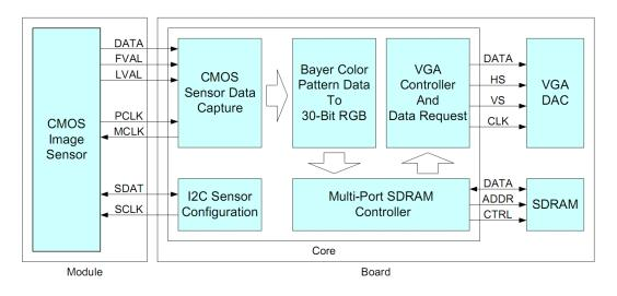
Figure 9.1: A block diagram of the Terasic camera system - from [55]
