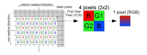
Figure 4.5: Color interpolation by using neighboring pixels to determine one full range RGB pixel - combined with figure from [56]
