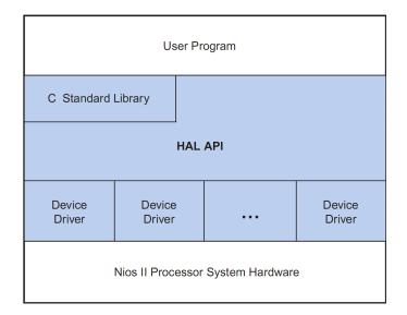
Figure 5.2: The layers of a HAL-Based System - from [20]
