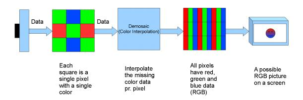
Figure 4.3: The process of transforming raw image data to viewable RGB image data
