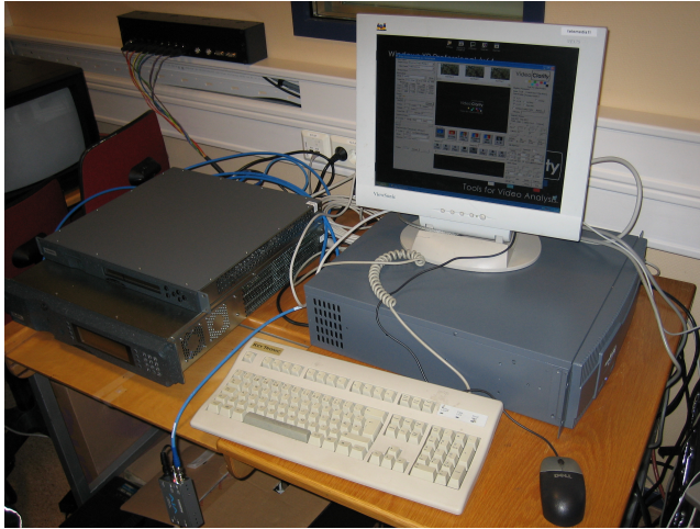
(a) The VQA system is located under the monitor. The decoder is hardware on top, on the left side of the picture. The encoder is below the decoder.
