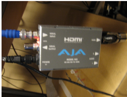
(b) The HD-SDI to HDMI converter used to play out from the VQA system on the monitor
