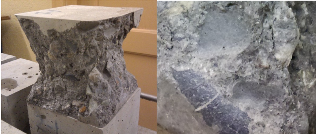
Figur 4.4: Referansebetong. Bruddform for terningene.
