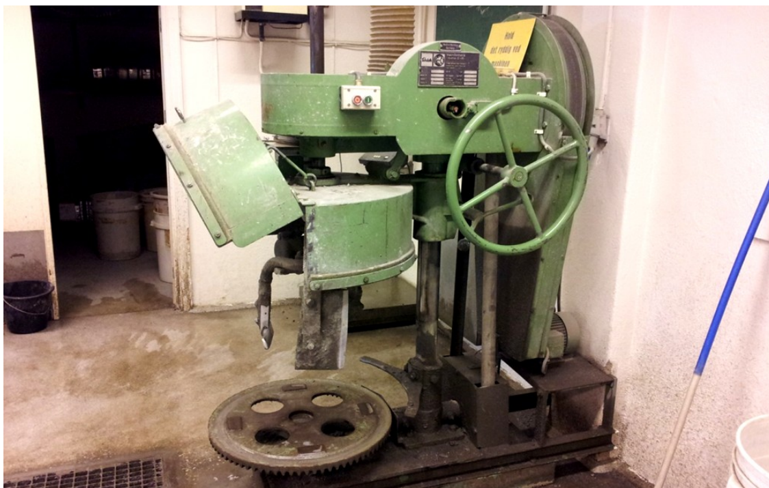
Figur 3.3: EIRICH SG1 50 liters tvangsblender
