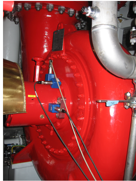
Fig. 3.3: Velometers mounted on the PB
