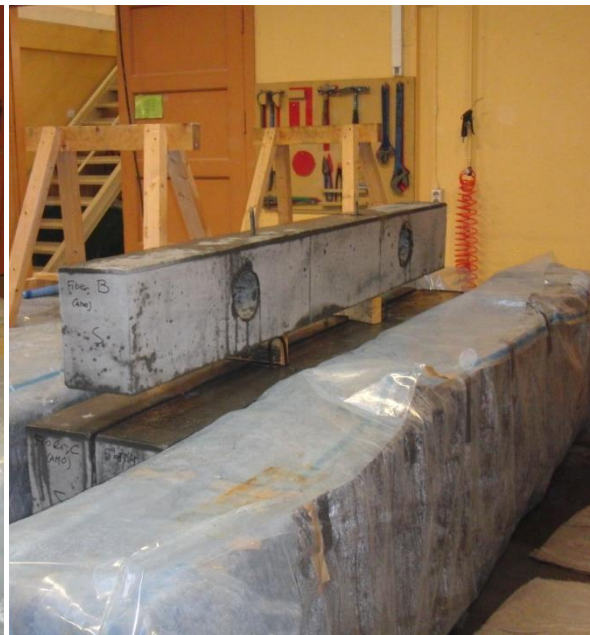
Figure 54: Beams piled for hardening
