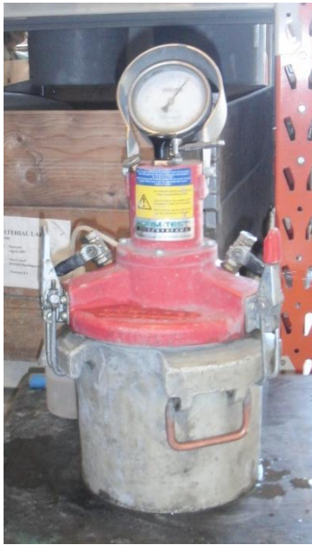
Figure 40: Air content measure, FTS-B 2020 apparatus
