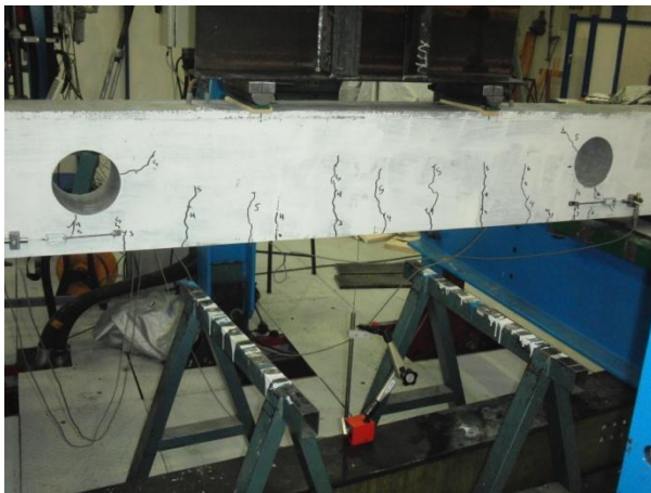
Figure 71: Crack development, beam A
