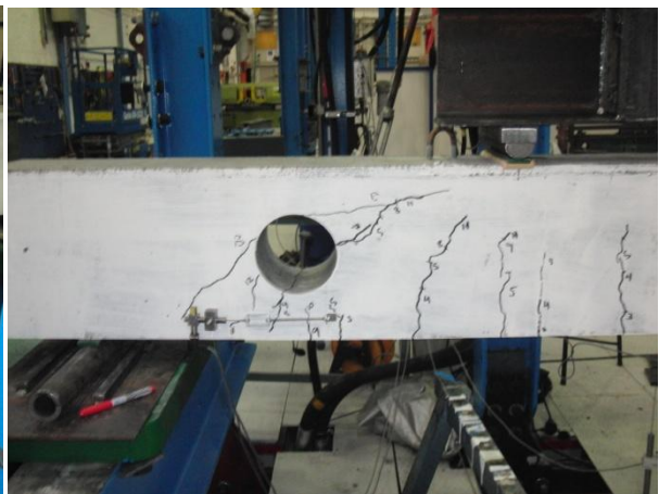
Figure 72: Close to failure, beam A
