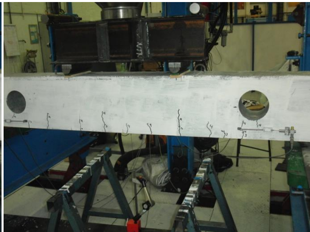
Figure 70: Crack development, beam A
