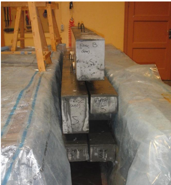
Figure 53: Beams piled for hardening
