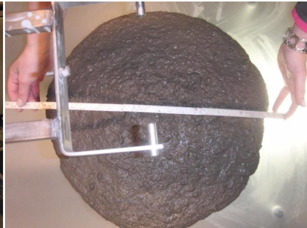
Figure 56: Measuring the slump
