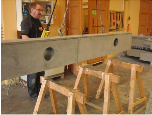
Figure 46: Beam A after removing the formwork
