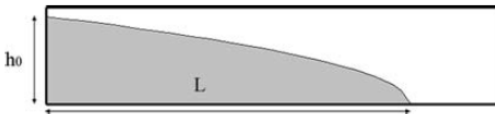
Figure 39: Flow of concrete in the LCPC-box (Roussel, 2007)
