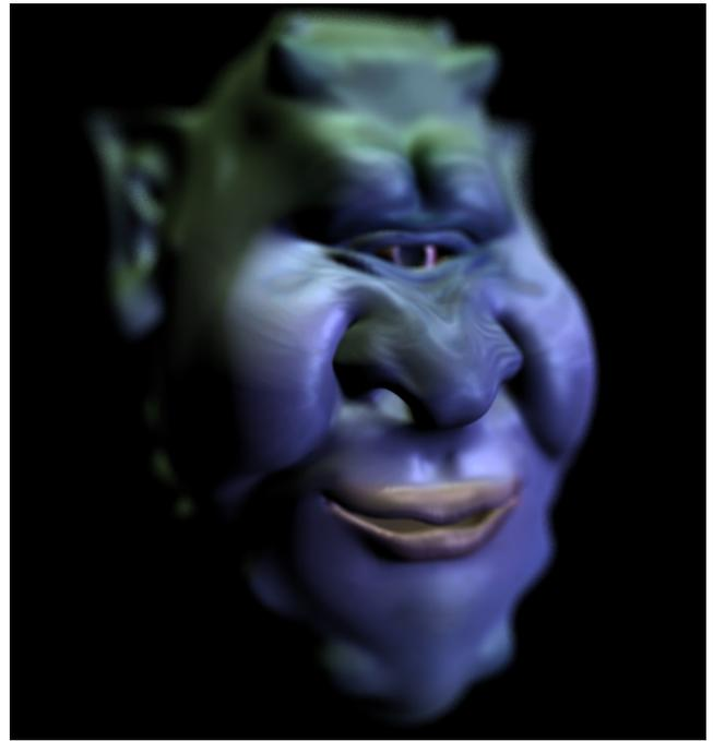
Figure 8: A 598 × 634 image of an animated character rendered with depth of field using a 256<sup>2</sup> (131,072 effective triangles) geometry image. 97,057,792 rays were evaluated in under 2 minutes.
