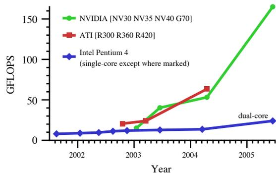
**Figure 1:** The programmable floating-point performance of GPUs (measured on the multiply-add instruction as 2 floating-point operations per MAD) has increased dramatically over the last four years when compared to CPUs. Figure courtesy Ian Buck, Stanford University.
