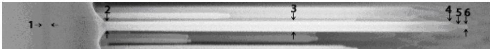
Figure 3.6: Example of the measurements done on the NWs in this study. (1) Thickness of Al marker, NW diameter at the bottom (2), centre (3) and top (6). The start and end of tapering at the NW tops is indicated with (4) and (5) respectively. The length of the NWs was measured from the kink (at (2)) and to the top of the Au particle (at (6)).
