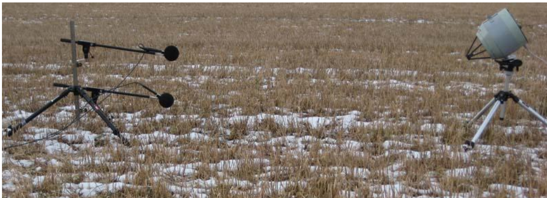
Figure 4.2: Ground impedance measurement setup at the simple test site.
