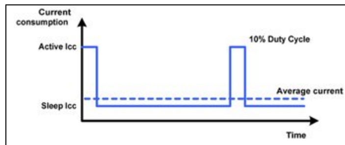
Figure 5.1 - Power Budget [11]. As the microcontroller is in sleep mode most of the time, the average power consumption is mostly dependent on the power consumption in sleep mode.
