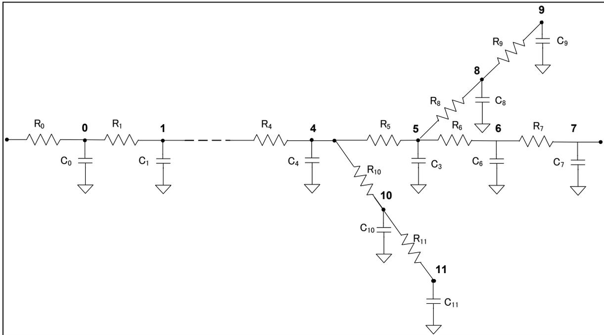
Figure 23. RC model of test path in [Tahoori 02]
