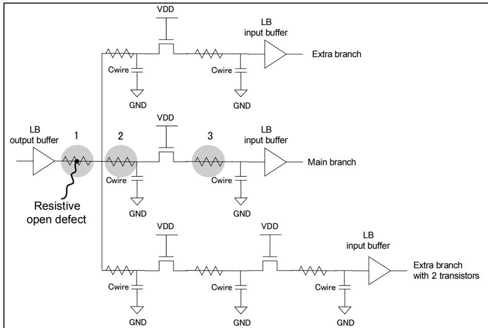
**Figure 8. SPICE setup and defect location (LB = logic block)**
