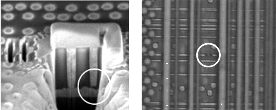
Figure 4. *Left*: incomplete contact etch (www.micromagazine.com); *right*: break on a net (www.ibm.com)
