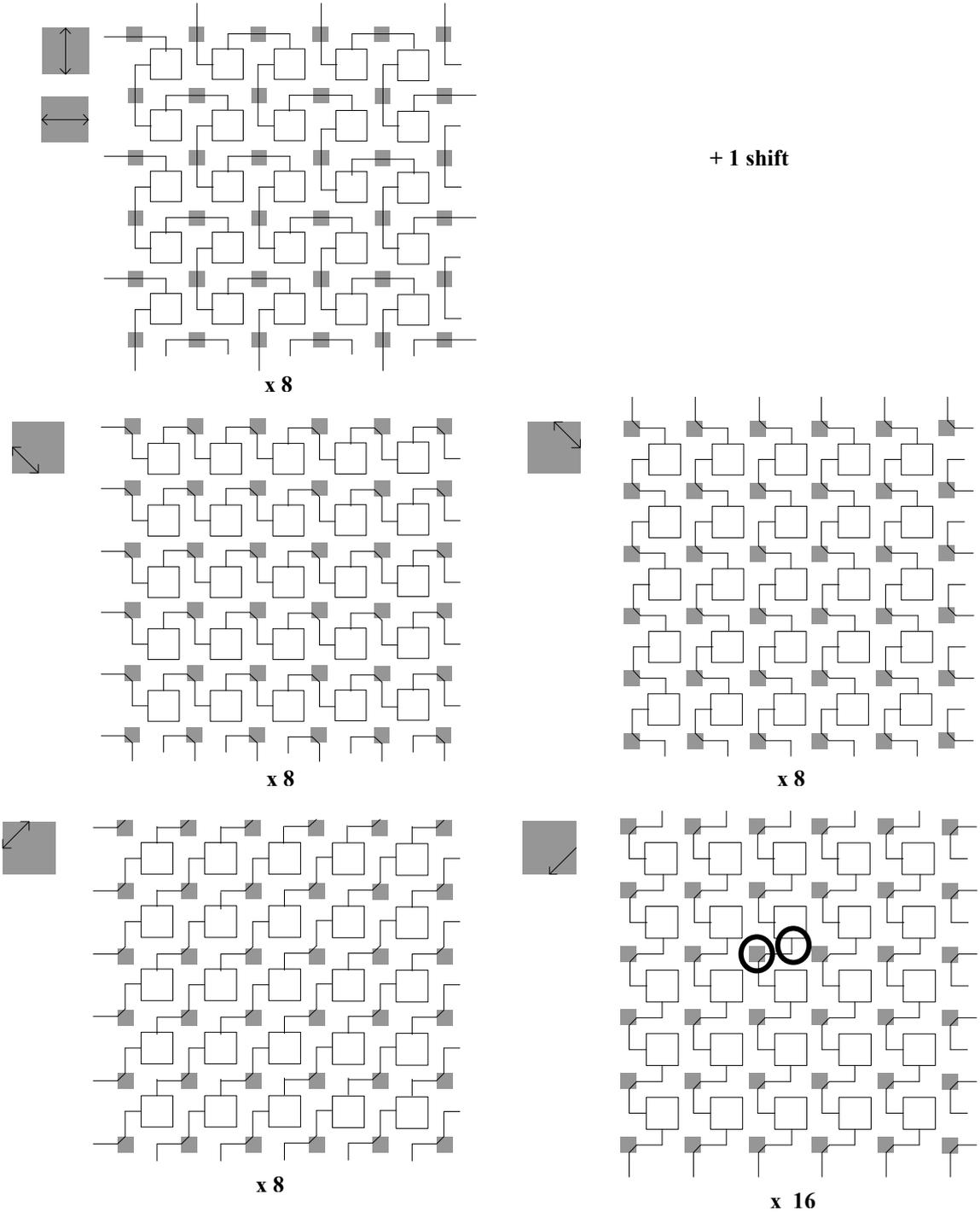
**Figure 22. Test configurations for XC4000 FPGA architecture**
