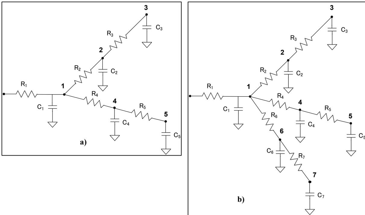
Figure 20. RC models of a) 2-branch test path and b) 3-branch test path)
