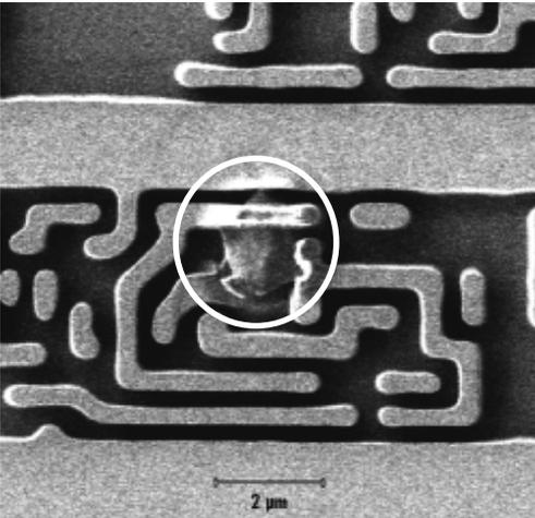
Figure 3. Short across several nets caused by a particle (www.micromagazine.com)
