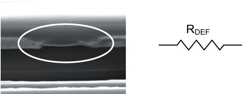
Figure 5. Closer view of the net break on Figure 4 and the circuit diagram symbol of the defect
