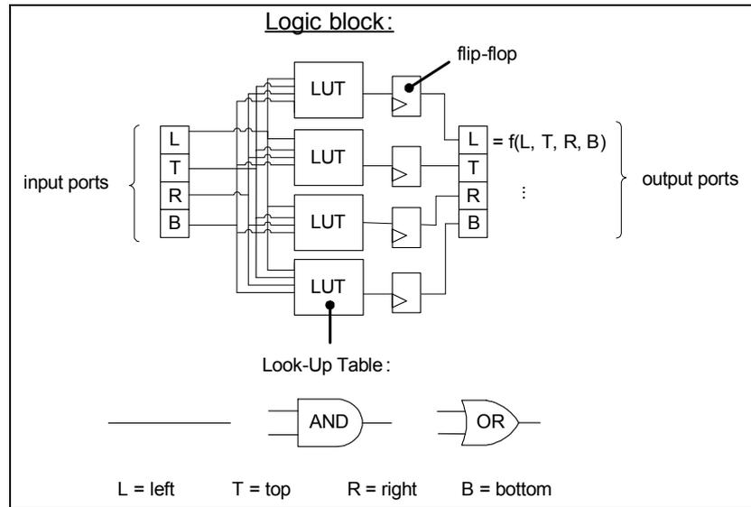
Figure 2. Logic block functionality
