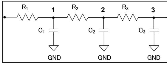
**Figure 19. 3-stage RC chain model of 1-branch test path**
