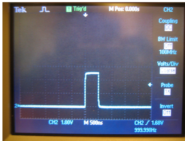
Figure 8.25: PCO 7120 output across a 1\ \Omega resistor. The voltage value is halved because of coax termination to the oscilloscope, making the real voltage 5 V. This corresponds to 5 A across a 1\ \Omega resistor.
