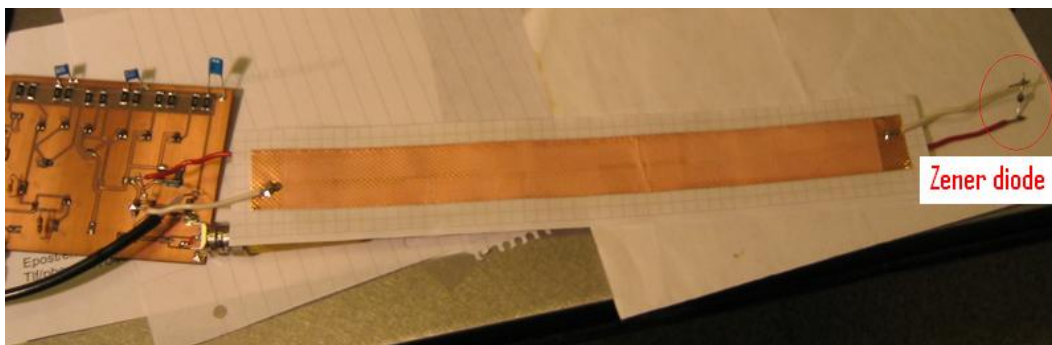
Figure 8.29: Output from PCB with laser equivalent zener diode mounted at the end of 30 cm long TP copper wires. Peak voltage of 396 mV corresponding to 2.4 A current magnitude. Pulse width of 500 ns.
