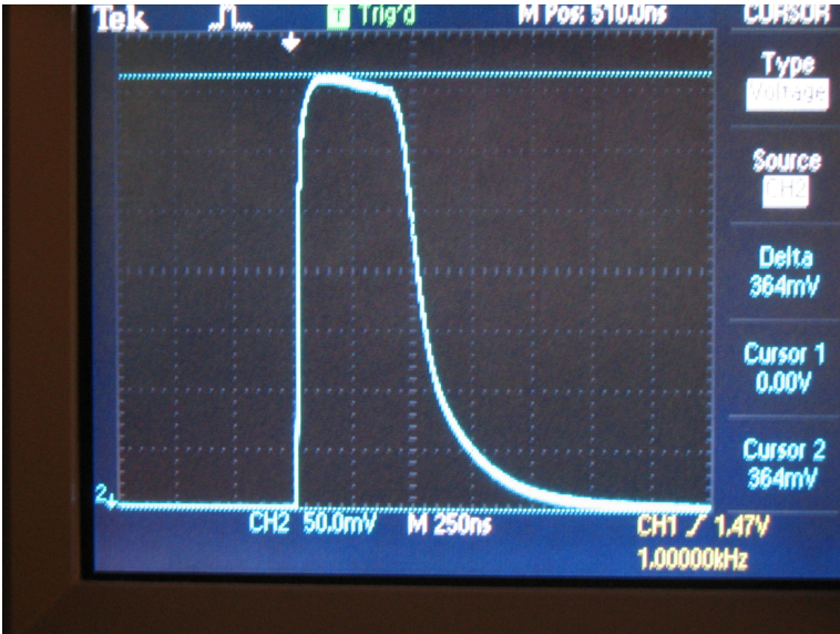
Figure F.38: Zener mounted on PCB. Current peak of 2.2 A
