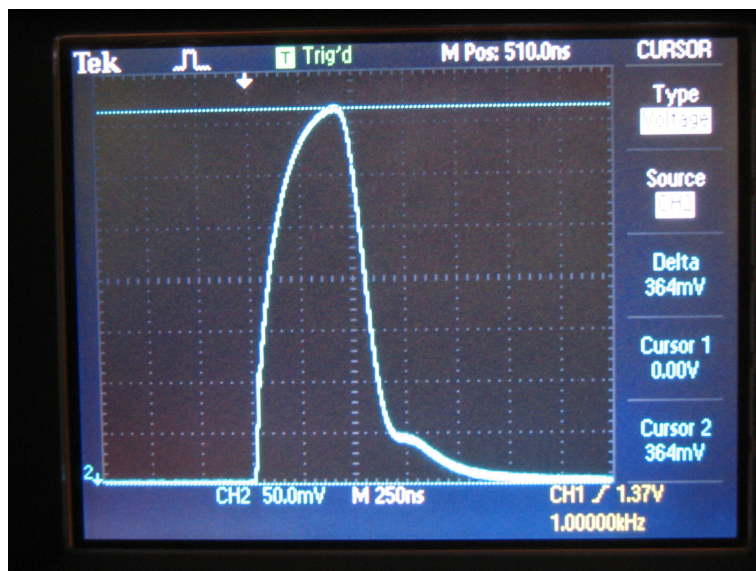
Figure F.40: Zener mounted with TP wires. Current peak of 2.2 A
