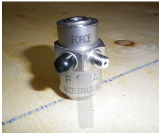
Figure 6.2: Accelerometer mounted using a double sided threaded stud
