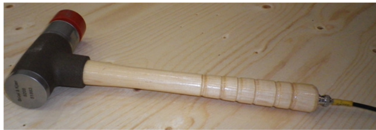
Figure 6.1: The modal hammer used for all experimental studies
