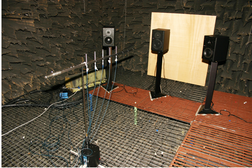
Figure 3.10: Frontreflector in anechoic room
