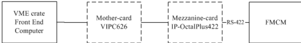
Figure A.3: Communication chain between the FCCM and the front end computer
