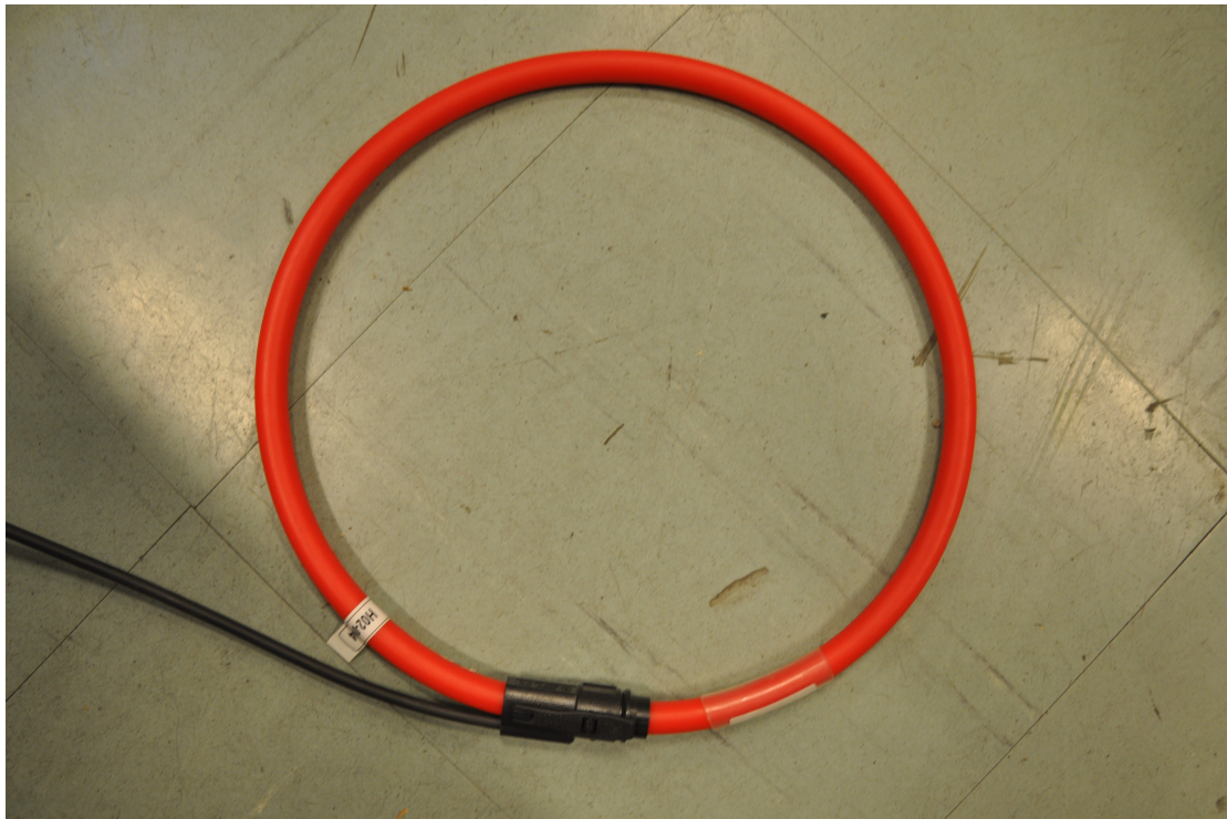
Figure F.15: One of the Rogowski coils used for current measurements with EL-SPEC.
