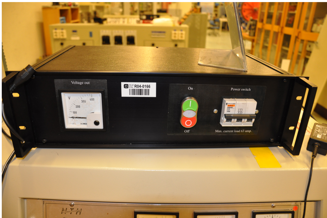
Figure F.12: Soft start equipment. An internal circuit containing resistance reduce in rush current, and disconnect the resistance after a few periods.
