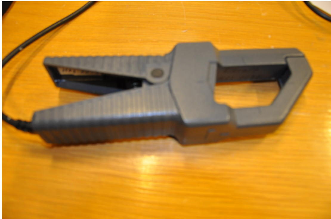
Figure F.14: Current clamp used for current measurements with oscilloscope and FLUKE.
