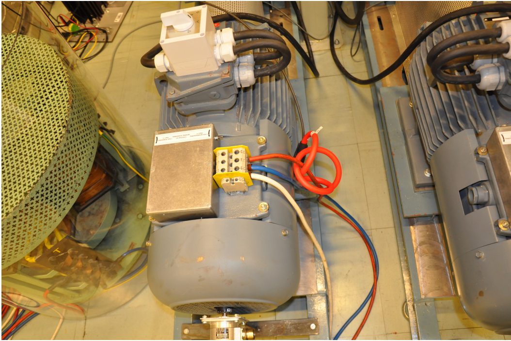
Figure F.5: Induction machine. Red, blue and white wire is connected to the rotor via slip rings, and rotor resistance is connected in the other end. One Rogowski coil is entangled three turns around the red conductor, as a control for rotor current.
