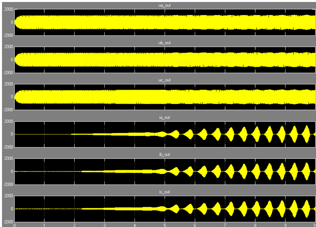
Figure 9.2: 1940 kVA generator system voltage and current in all three phases a, b and c.
