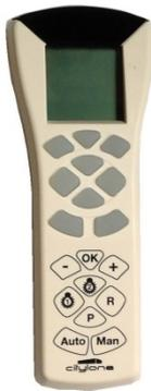
An infrared configuration remote controller (SL-TP-T) can be added to your installation in order to parameterize your controllers.
