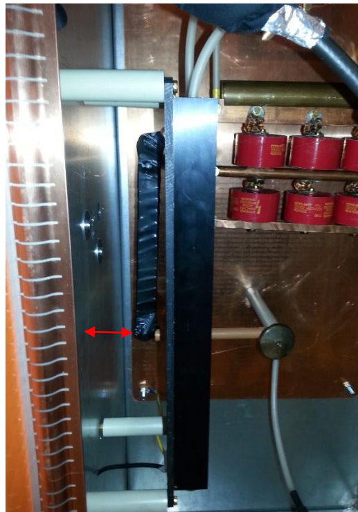
Figure 46 - Fast switching setup showing a critical distance from the grounded cabinet to a HV connection wrapped with semiconductive tape to avoid corona
