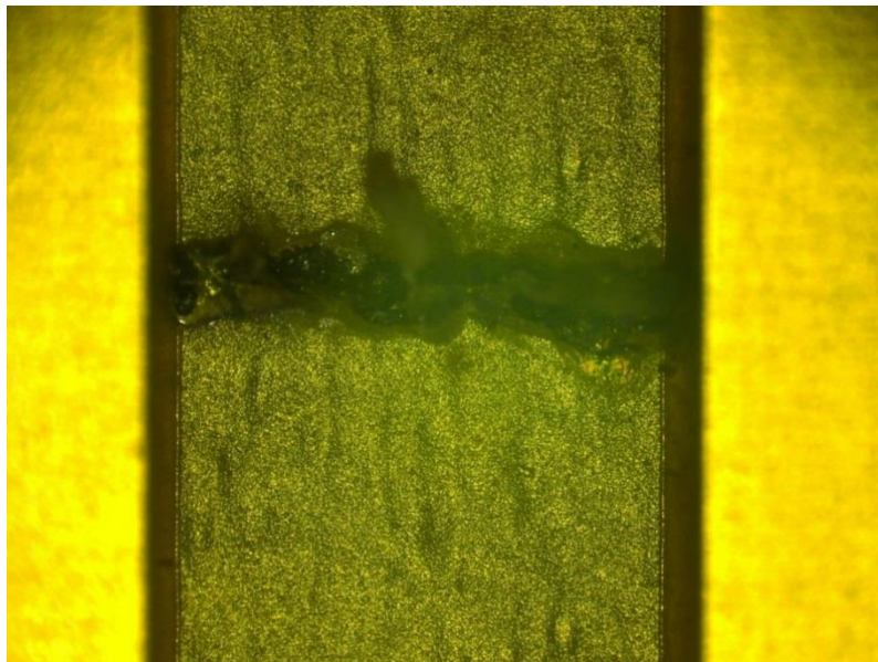
Figure 32 - Surface breakdown across the trench when the board had Parylene surface cover.
