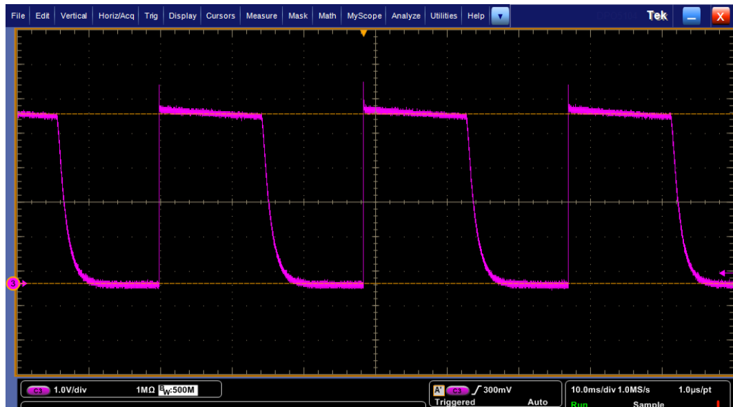
Figure 35 - Time response waveform of fast turn-on switching voltage across the test object
