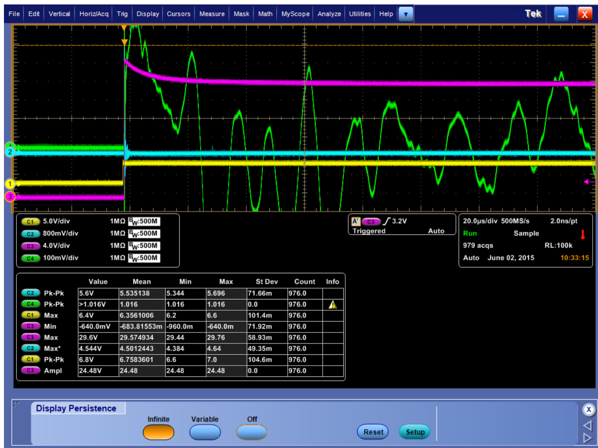
Figure 34 - Circuit response with persistence from 25 kV fast switching (3) showing the constant noise for the acoustic (4) and light signals (2)
