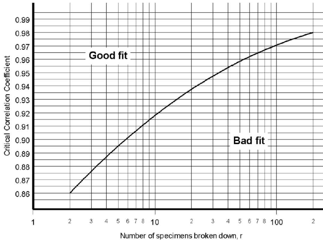
Figure 58 - Plot to check the goodness-of-fit of a two-parameter Weibull distribution
