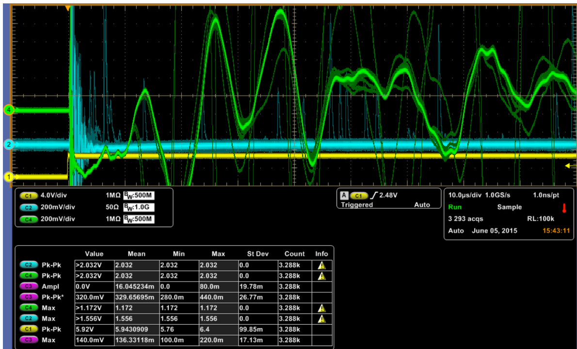
Figure 42- Nytro without cover at 27kV negative fast switching: Persistence shot with PD light signals appearing close to the voltage switching edge and extensive correlating acoustic signal after 20μs
