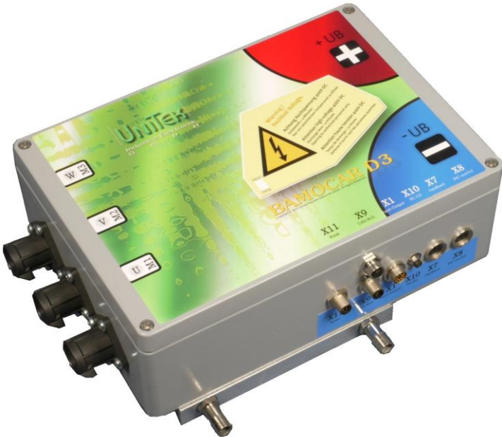
Figure 1.11: Bamocar d3 voltage source inverter.
