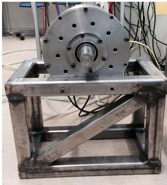
Figure 9.6: Initial PM motor test rig, front side.
