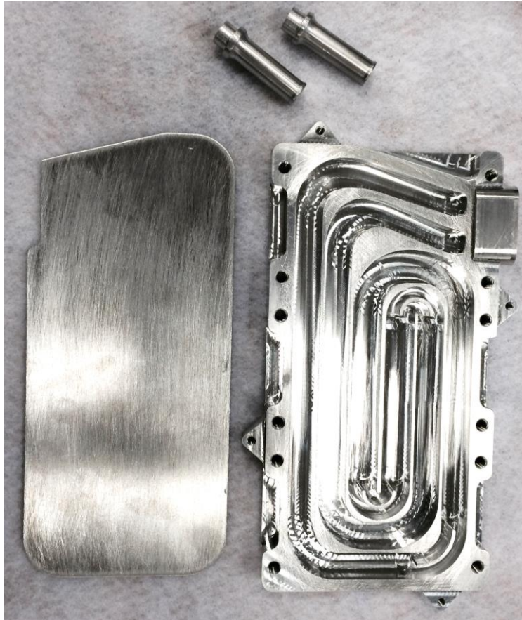
Figure 8.4: Aluminum heatsink with base plate and nipples.
