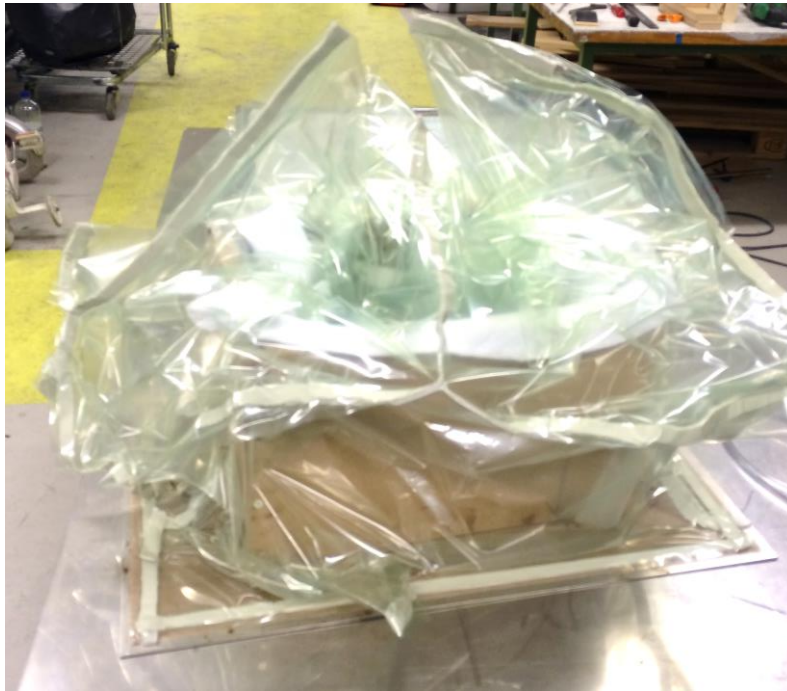
Figure 8.7: Carbon fiber casing vacuum packing.
