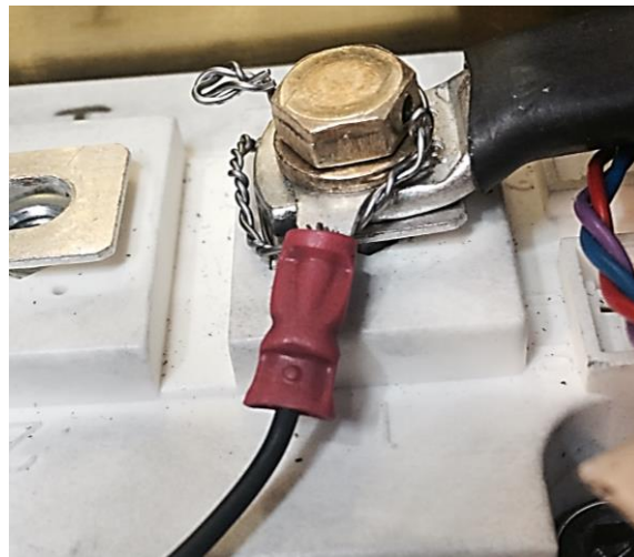
Figure 8.11: Positive locking of the AC terminal contacts.
