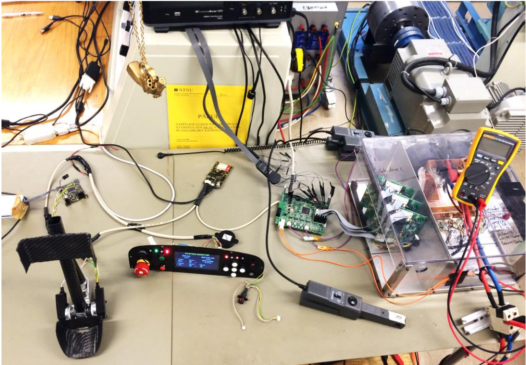
Figure 9.11: Test setup with torque pedal, ECU and dashboard.
