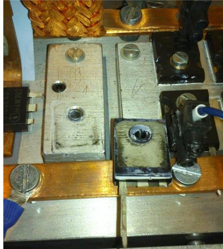
Figure 6.7: Destroyed diode and heat sink
