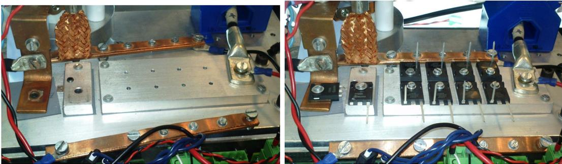
(a) Bypass components removed
