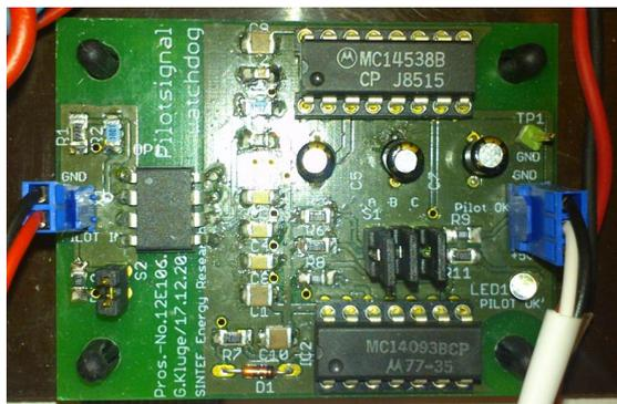
Figure 5.17: SINTEF hardware watch dog card
