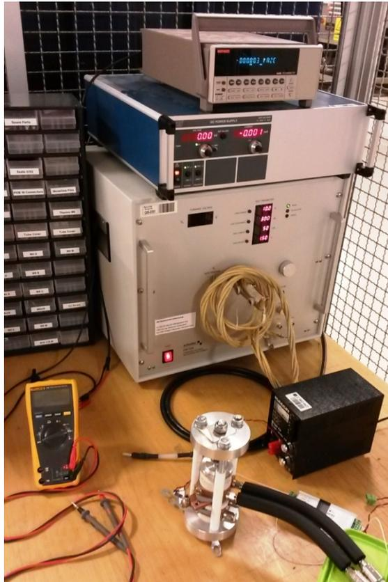
Figure 5.19: Single chip clamp and characterisation equipment
