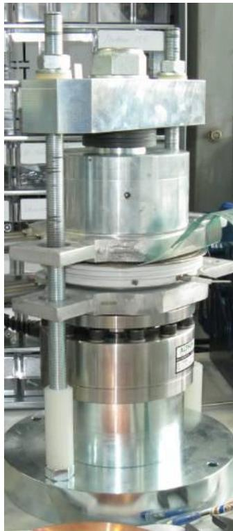
Figure 2.9: Clamping device for press-pack IGBT
