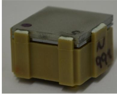
Figure 5.10: Press-pack IGBT chip
