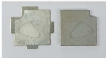
Fig. 4: Detail of mark between silver and molybdenum
