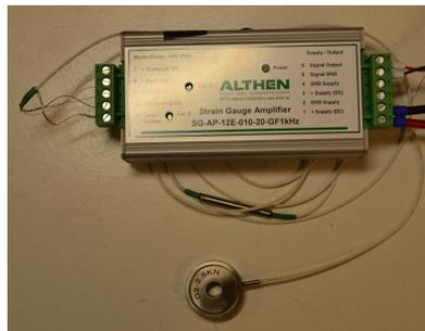
Figure 5.9: Pressure sensor with measure module
