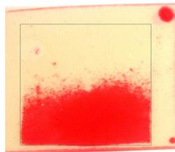
(a) Force distribution with initial collector contact
