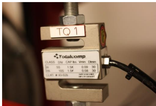
Figure 7-5: Torque sensor measuring torque developed by the PM-machine M-3
