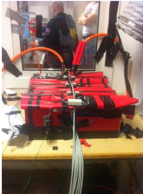
Figure 7-1: Setup of accumulator during water – brake testing.
