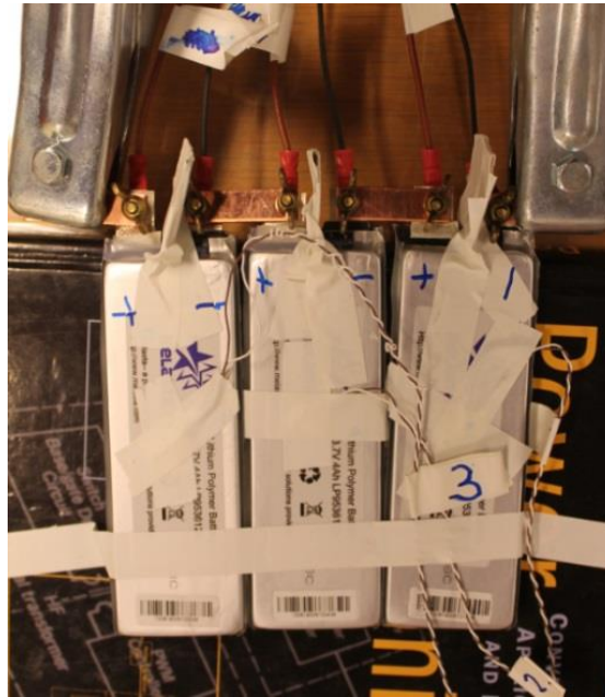
Figure 8-2: Connection of battery cells during tests A-1 and A-2.
