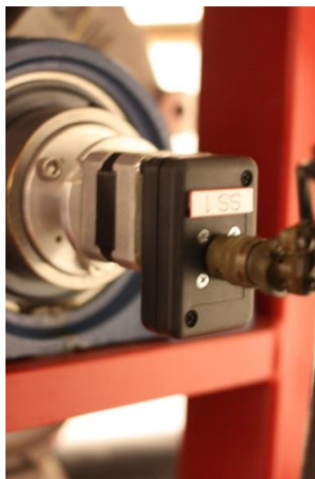
Figure 7-6: Speed sensor that measures the speed of the water brake drive shaft.
