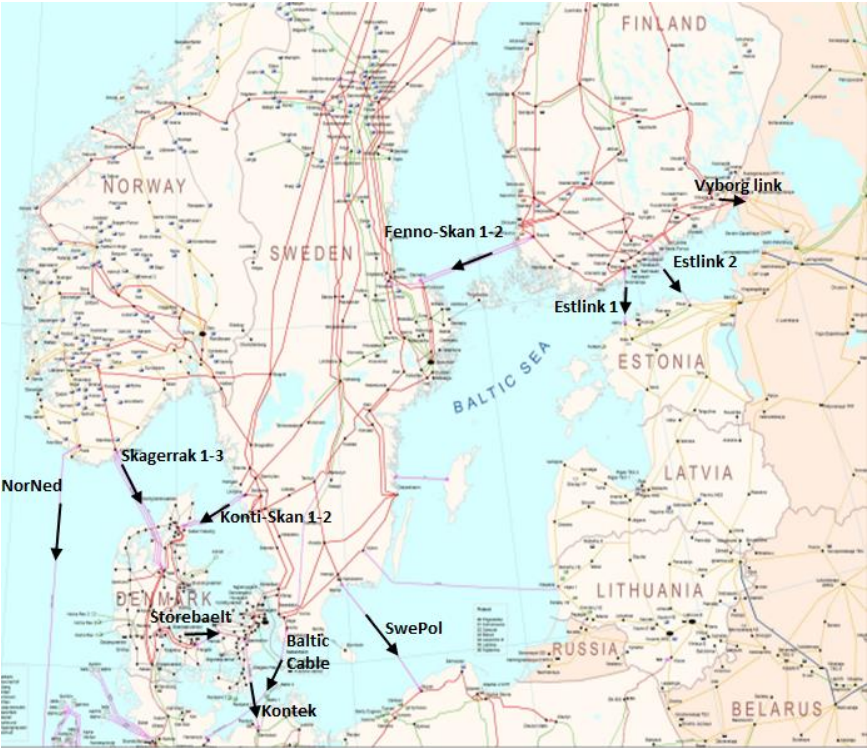
Figure 3.1: HVDC-cables overview connected to or within the Nordic Synchronous area. (Regional Group Nordic, 2014).
