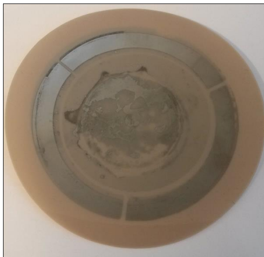
Figure 5.3. ASTM specimen with damaged/vanished electrodes. The aluminum is intact at contact points with external measurement- and guard electrodes.
