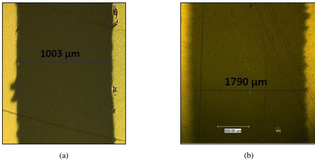
Figure 5.6. Gap length of the ASTM specimens. (a) Minimum gap length (specimen no. 4) and (b) maximum gap length (specimen no. 1).
