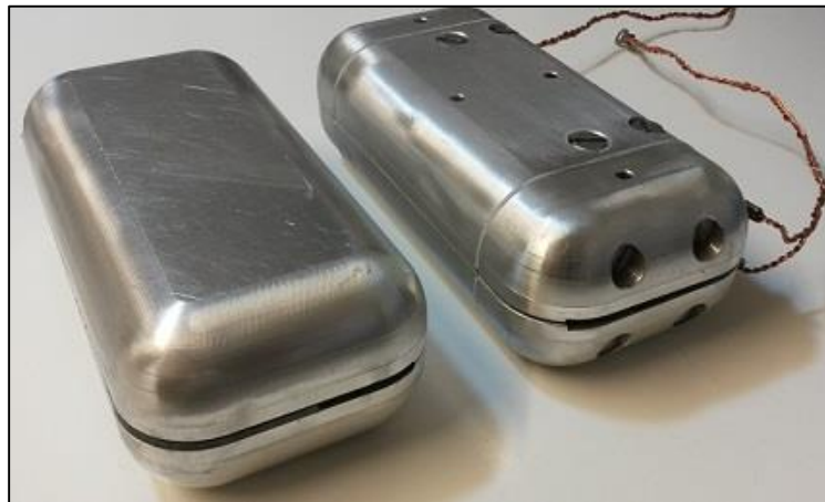
Figure 3.7. Final design for the external electrodes for the Alternative specimens. The wires are for grounding the guard electrodes.
