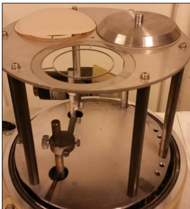
Figure C-3. ASTM specimens, electrode rings and weights mounted in the matrix prior to evaporation.
