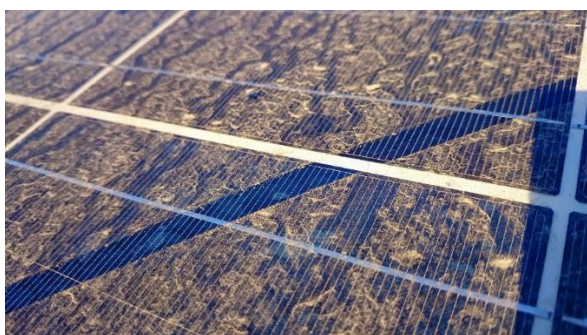
Figure 77 - Shading due to soiling. Shot at 19th of November 2014. Photo by Eirik Oksavik Lockertsen.
