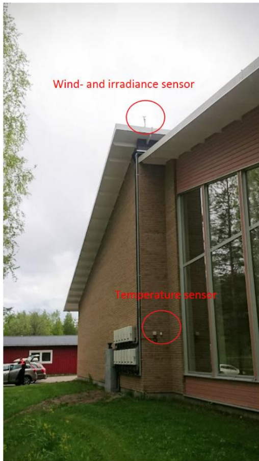
Figure 98 - Placement of the Acusticum temperature-, wind- and irradiance sensors. Photo by Eirik Oksavik Lockertsen.
