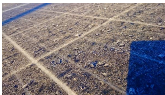
Figure 78 - Shading due to frost. Photo by Eirik Oksavik Lockertsen.
