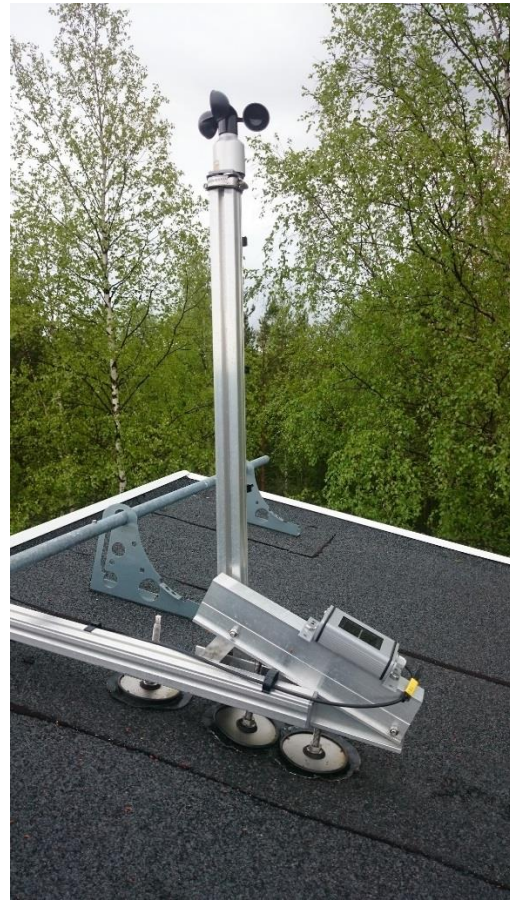
Figure 99 - The Acusticum wind- and irradiance sensors. Photo by Eirik Oksavik Lockertsen.
