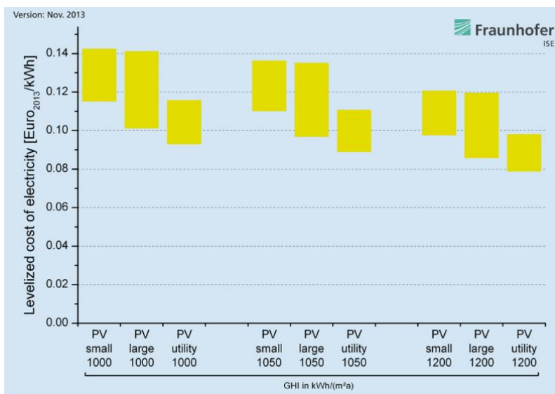
Figure 13 - LCOE for small (households), large (business partnerships) and utility size PV systems for different GHI values [1, 15].
