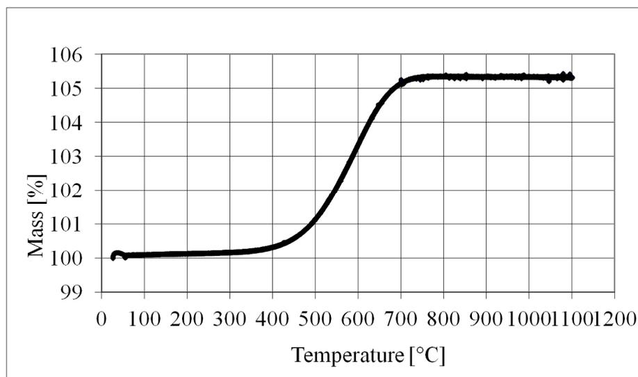
**Figure 3.** Thermogravimetric analysis of pure Inco 255 nickel powder in air.
