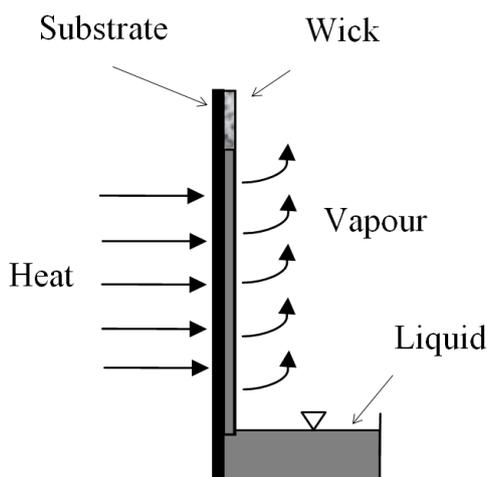
**Figure 1.** A flat wick attached to a solid substrate subject to a uniform heat flux causing liquid evaporation from the free wick surface. Liquid (condensate) is pumped by the wick from a reservoir at the bottom of the wick. The experiments utilized to characterize the wick in this study were performed without the heat addition and without the solid substrate.
