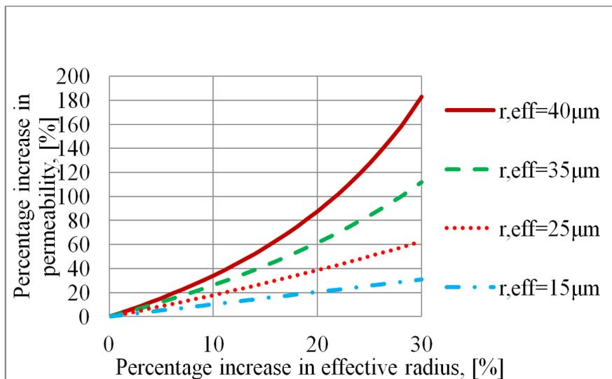
**Figure 10.** Pore former evaluation plot for  $H = 0.1$  m and heptane at  $20\text{ }^{\circ}\text{C}$ .
