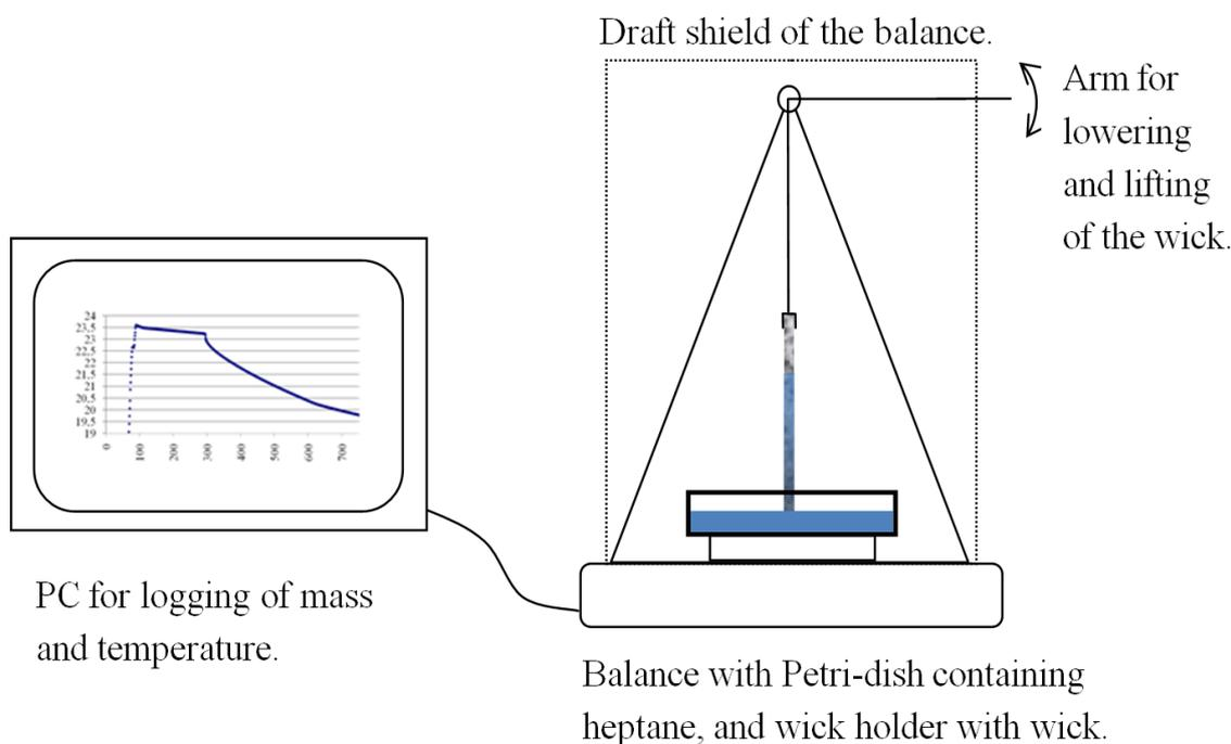
**Figure 2.** The rate-of-rise setup.
