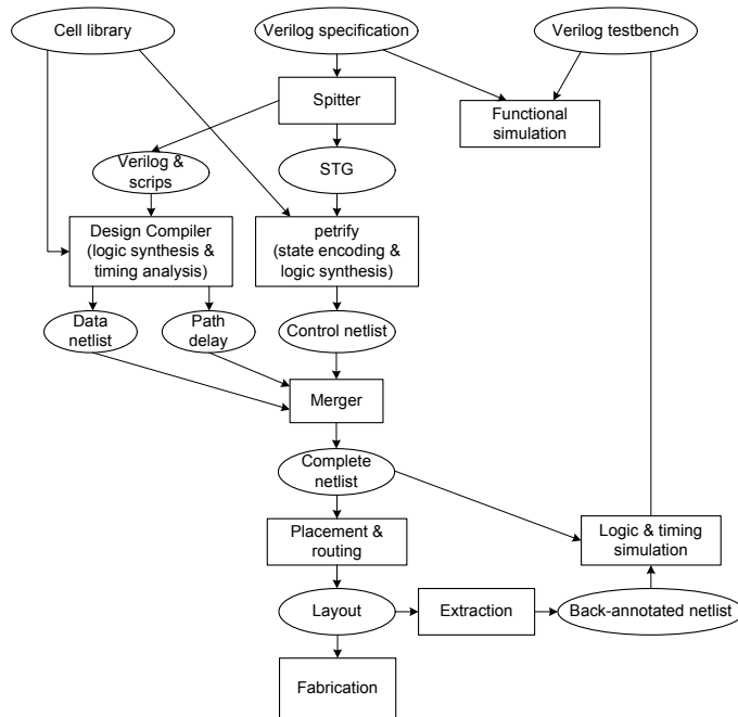
Figure 5.4: Block diagram of Pipefitter synthesis flow. Based on a figure in [9]
