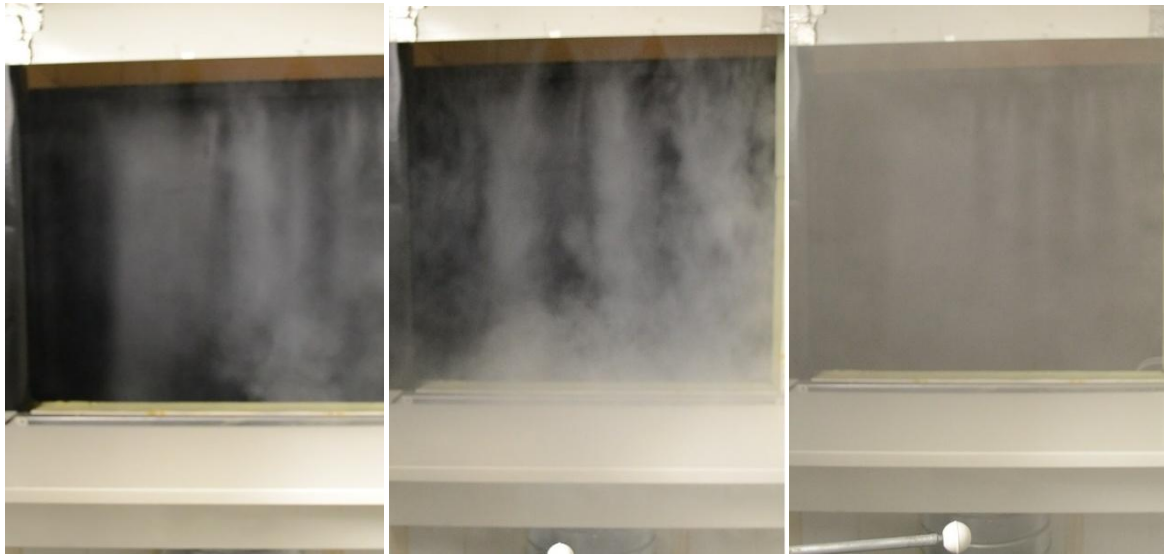
Figure 41. The flow of smoke gas, visualized for case when q_{sup}=173 \text{ m}^3/\text{h} q_{exh}=660 \text{ m}^3/\text{h} effective area =0.08 \text{ m}^2 a) beginning of smoke test b) center of smoke test c) end of smoke test
