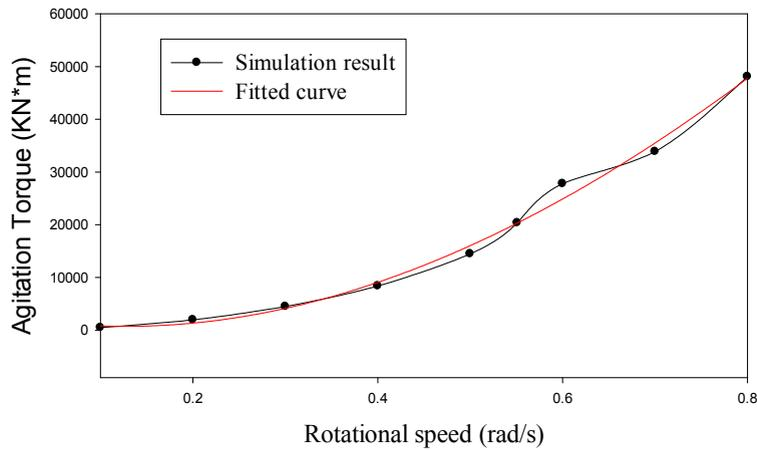
**Fig 4:** Relationship between rotational speed and torque
