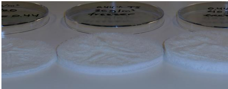
Figure 42: Thickness variation of filters with grammage of 20, 30 and 40 \frac{g}{m^2} , respectively. All filters in the image has the same dry weight content of 0.44%.
