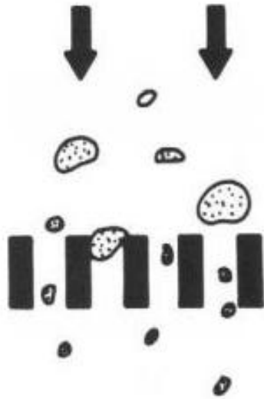
Figure 6: Filtration by surface straining where larger particles are deposited on the filter surface.
