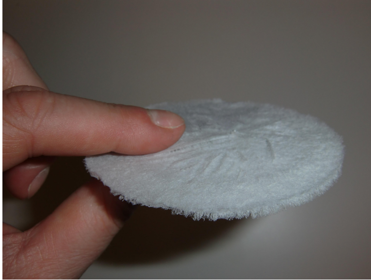
Figure 41: NFC filter which has been frozen in a deep freezer followed by vacuum drying.
