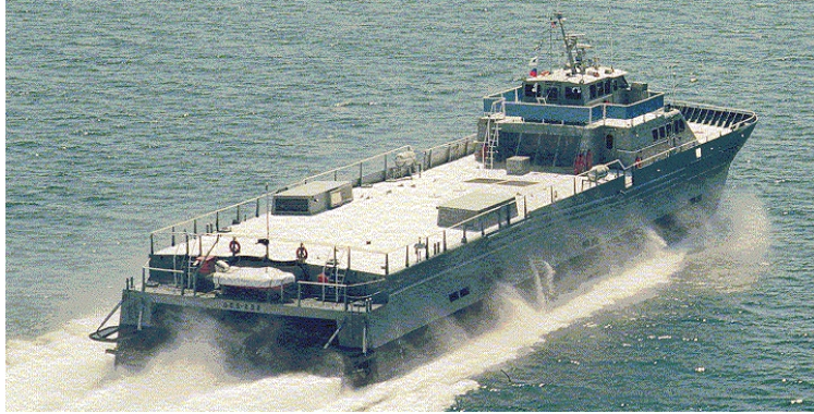
Figure 1.12: The SES 200 had a range of 3000 miles at 25-30 knots without having to refuel.
