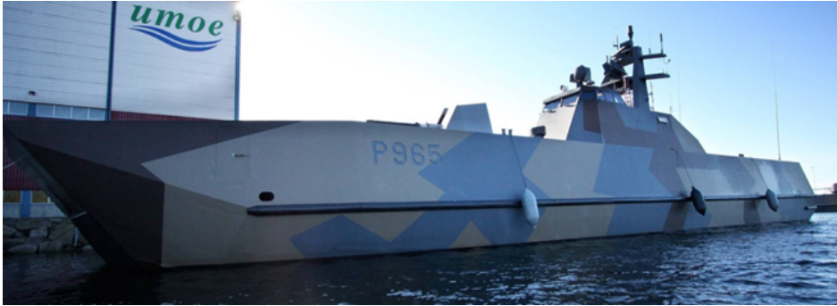
Figure 1.14: The Skjold class, maximum speed of 60 knots+ and overall extreme performance, by courtesy of UM.
