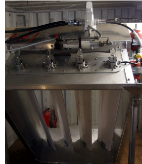
Figure 5: A vent valve assembly from a full-scale system bench-test. Courtesy of Umoe Mandal.
