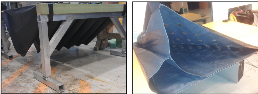
Figure 1.20: The scaled flexible seals.
