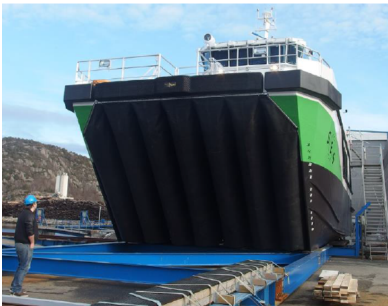
Figure 3.2: The Wave Craft prototype seen from the front. The bow skirt is visible. Photo: Umoe Mandal.
