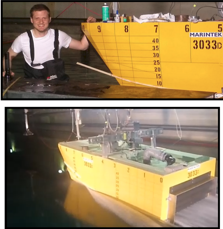
Figure 1.22: Resistance and drag tests in calm water performed in the Ship Model Tank.
