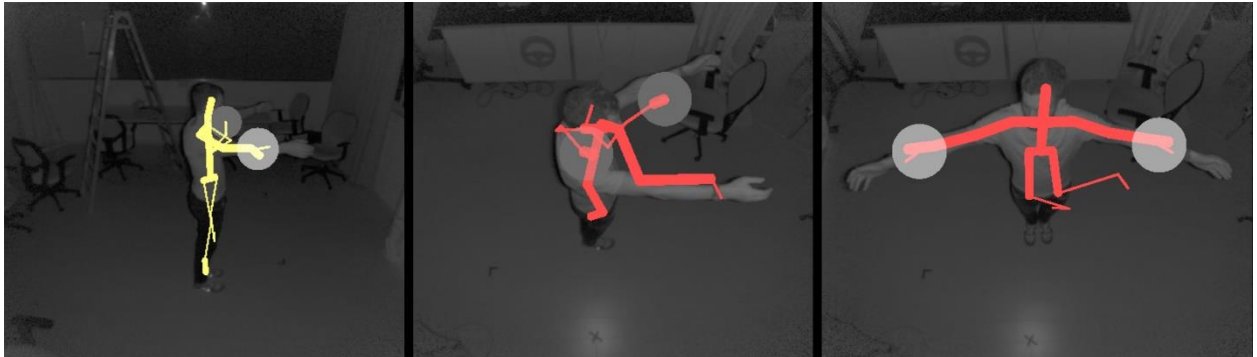
Figure 4.3 Microsoft Body Tracker. Even though the Microsoft Body tracker achieves a tracking result, the tracking may be far from the ground truth. Left: Tracking at -30 degrees. Middle and Right: Tracking at -60 degrees
