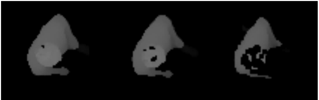
Figure 8.6 Index in sorted kernel. The filtered results from choosing different indexes in the sorted kernel. Left: Index 2. Middle: Index 4. Right: Index 8. The person in the frame has shiny black hair and we see that if a high index is chosen depth data will be lost.
