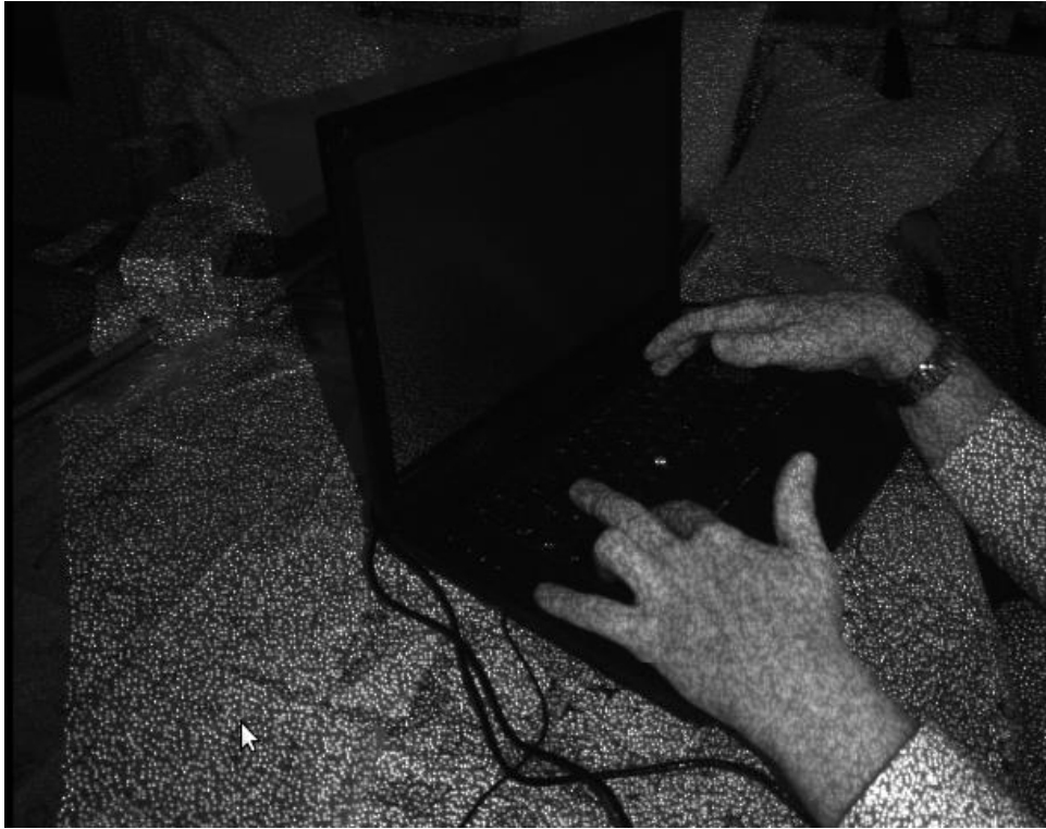
Figure 3.4 The pattern of infrared dots emitted by the Kinect v1. Source: ("Kinect," n.d.)
