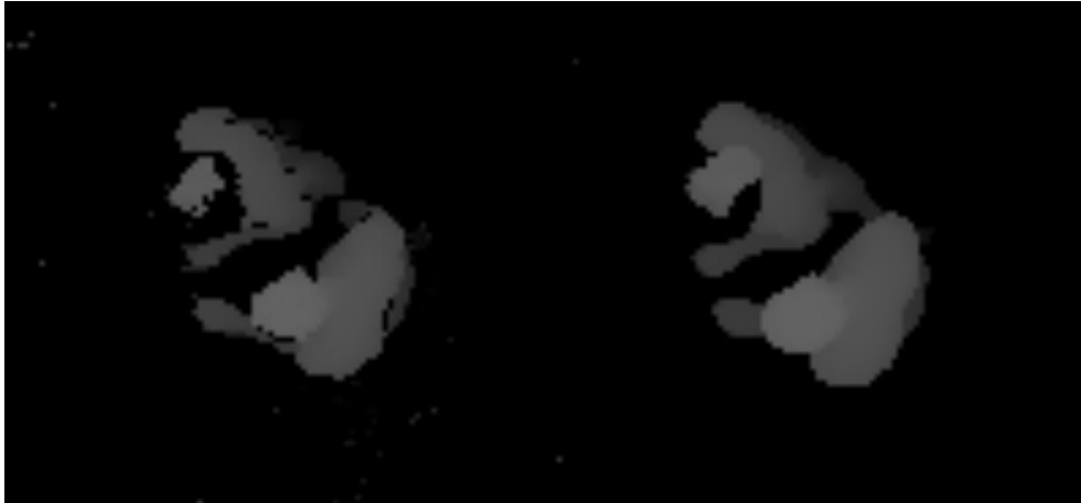
Figure 8.7 The foreground area in the frame before (left) and after (right) median filtering.
