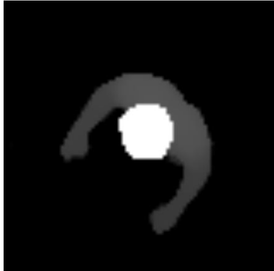
Figure 8.11 Head blob. A head blob after growing region with the connected-component algorithm and validation.
