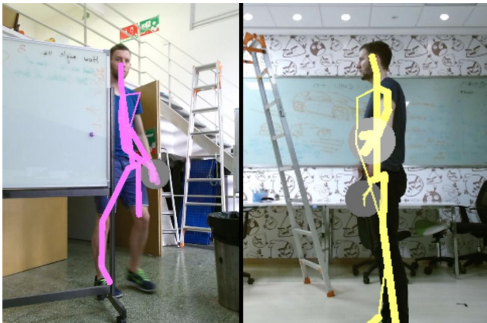
Figure 4.1 Occlusion: Left: Normal occlusion. Right: Self-occlusion. The tracking results of Microsoft Body tracker has challenges matching the ground truth.
