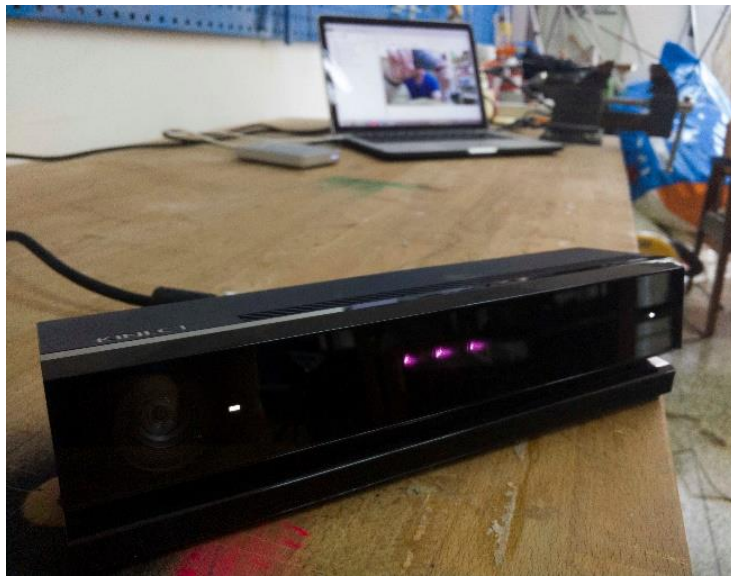
Figure 3.5 The three laser diodes (purple) in the Kinect v2.
