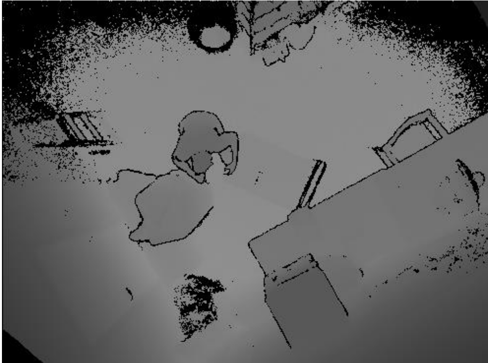
Figure 9.4 Flying pixels can be seen along the edges of objects.
